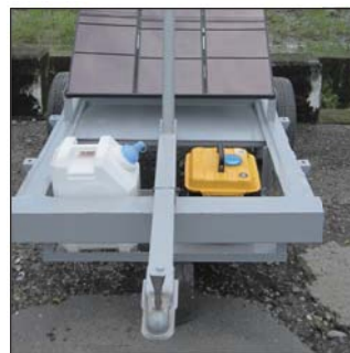
Gas tank / Gas generator
